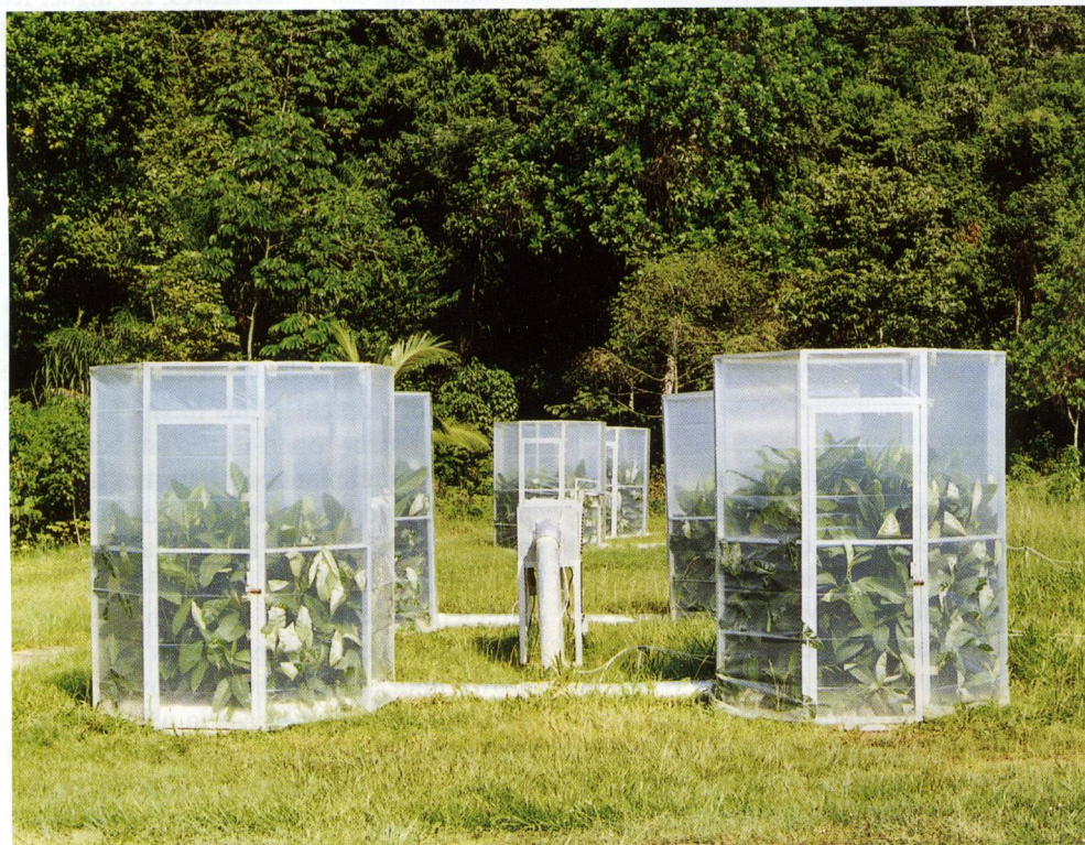
Fig. 1. Open-top chambers with communities of Ficus insipida and Virola surinamensis during the final part of the 16 week experiment. Left, community at ambient CO 2 ; right, community at elevated CO 2 .
